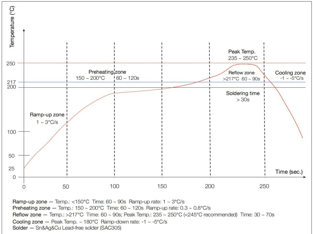
**The module Must go through 125°C baking for at least 9 hours before SMT AND IR reflow process!**
